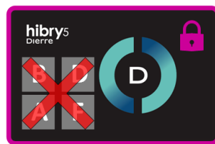
Figure 6.8: The purple NFC key is formatted: all internal cryptographic data is erased and the key will no longer be able to open any door. The key memory is cleaned and can once again store credentials for access to about 25 doors.
